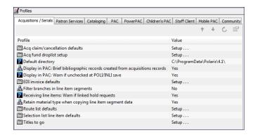
Select Filter branches in line item segments and select Yes or No. If this filter is set to Yes, it also filters branches in the bulk add process. For more information on the implications of setting this filter, see "Filtering Branches in Line Items" on page 93.
