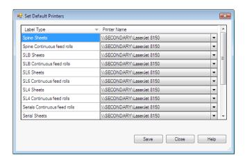
3. For each label type that is enabled and appears in the Label Type column, select the default printer in the Printer Name column.
